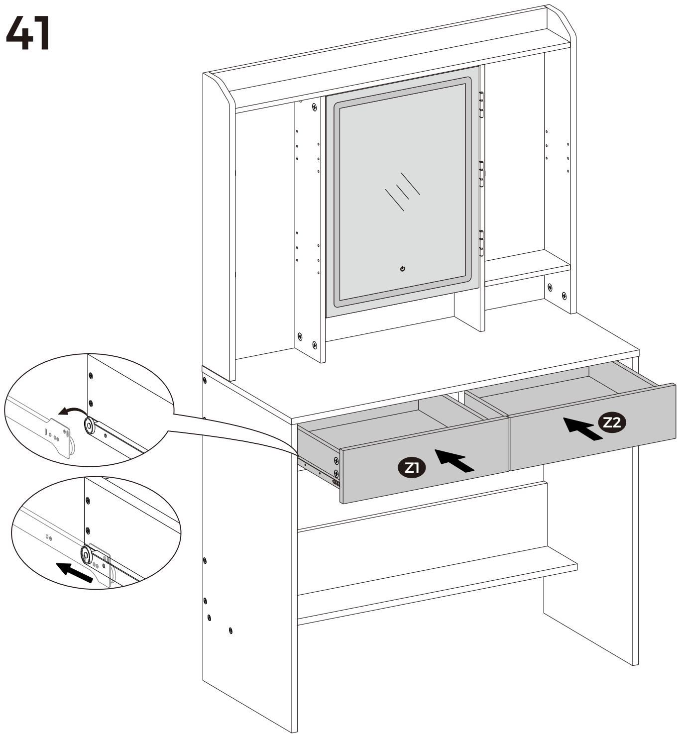
**EN** The gap between the two drawers is large: Switch position of the drawers; left drawer goes to the right, right drawer goes to the left.
