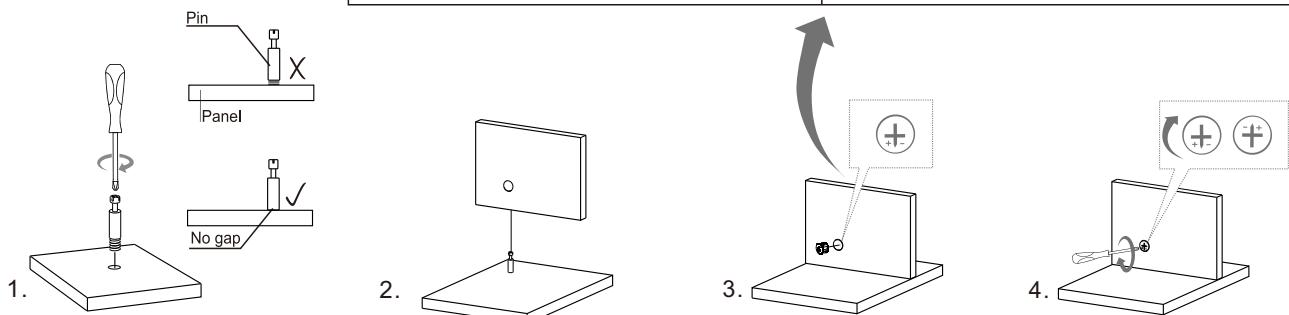
**1** Note : Please use a manual screwdriver or an electric drill on a low-torque setting to prevent damage to the panels.
