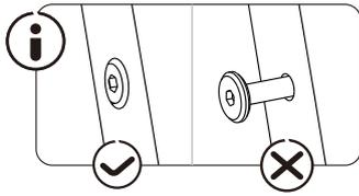
**EN** • Note: Securely tighten all screws and regularly check during use.
