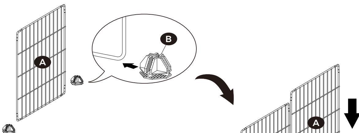
**EN** Before the next step, please check and make sure that all the panels are inserted into connectors entirely.
