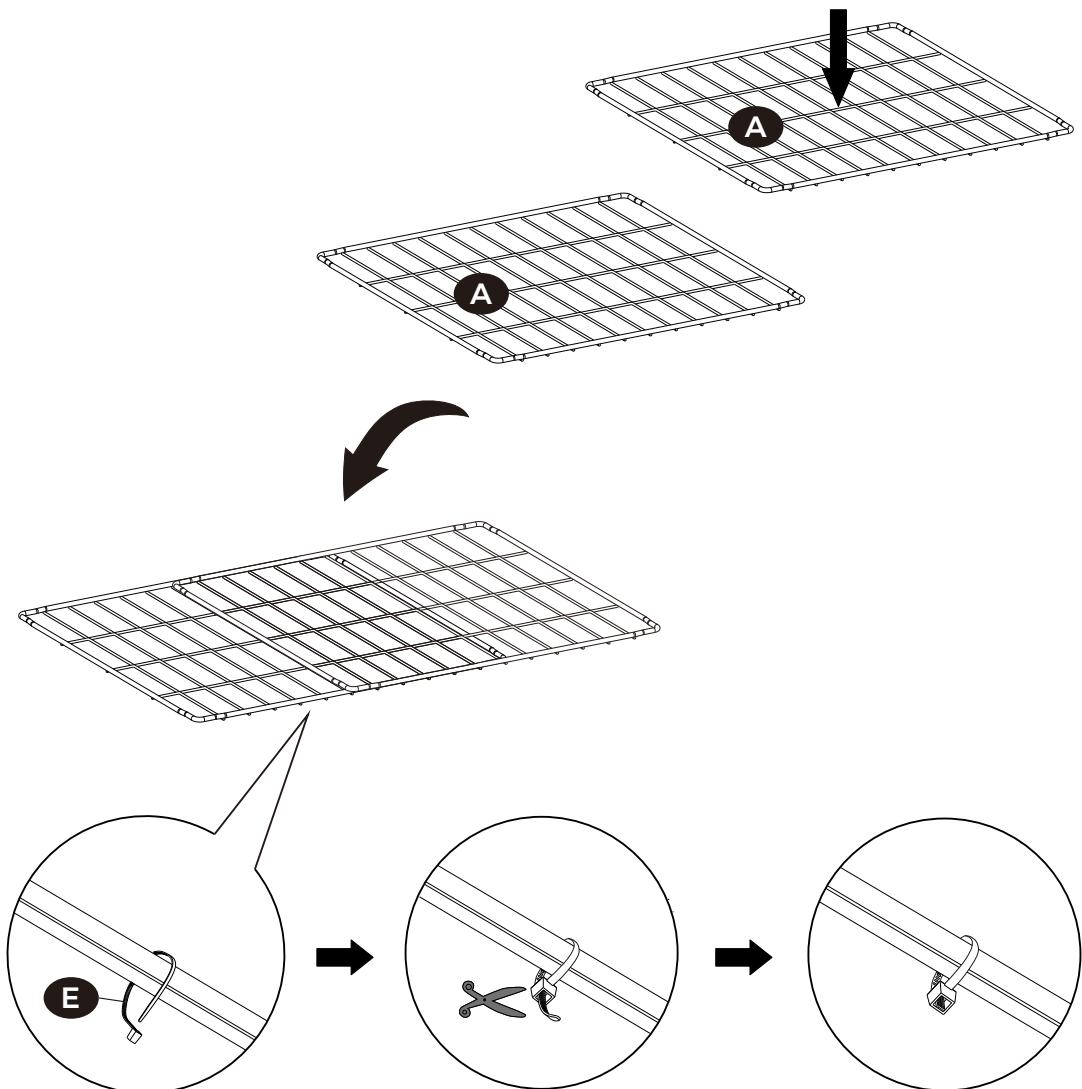
**EN** As shown in the picture, attach the two wire mesh panels together with cable ties.
