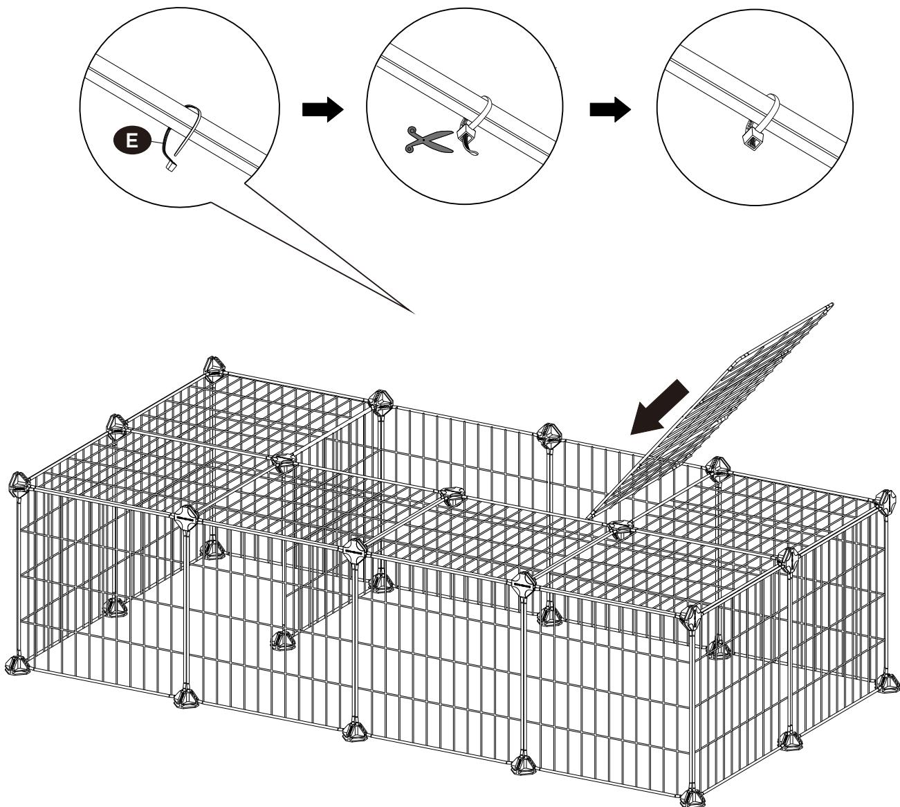
**EN** Insert cable ties into the 2 connection corners to attach the wire mesh stairs and second-floor platform together.
